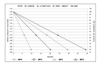
should be administered. However, it is advisable to conduct an inspection and Open Circuit Voltage (OCV) check after 12 months and recharge if the OCV is less than 2.10 volts per cell. When stored at temperatures in excess of 30 °C (86 °F), the battery should be OCV-checked every six months. The graph above shows the relationship between temperature, storage time and OCV.
